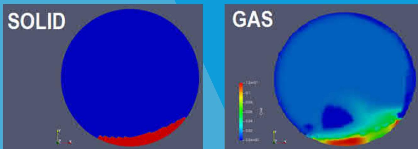
The numerical model allows evaluating the heat exchange between the organic substrate and the gas-liquid fraction, as well as between the reactor and the organic matrix. The simulation solves the solid disappearance through thermochemical kinetic models.
