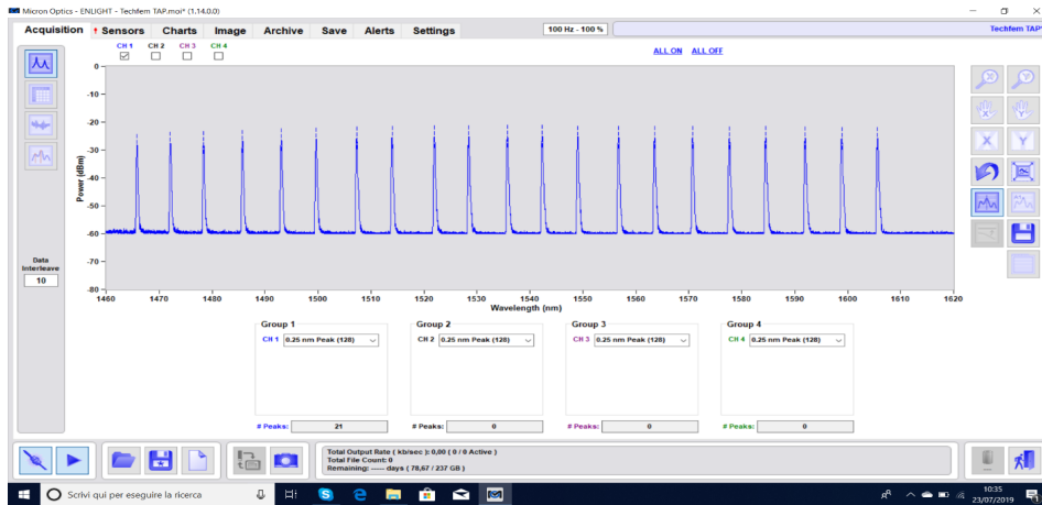
Fig 8: Spectra peaks of FBG sensors Bragg Wavelength
